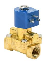
GC Valves solenoid valve, 2-port (2-way), 2-position, N.C., brass body, Viton seal(s), 1/2in female NPT inlet(s), 1/2in female NPT outlet(s), Cv=3.3, 1 psi minimum operating pressure, 120 VAC operating voltage, 18mm DIN style wiring plug.
