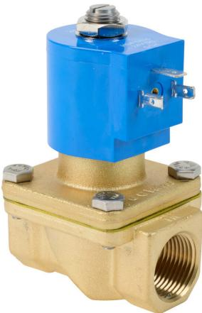
GC Valves solenoid valve, 2-port (2-way), 2-position, N.C., brass body, Viton seal(s), 3/4in female NPT inlet(s), 3/4in female NPT outlet(s), Cv=6.7, 0 psi minimum operating pressure, 24 VDC operating voltage, 18mm DIN style wiring plug.
