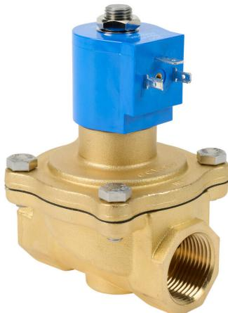
GC Valves solenoid valve, 2-port (2-way), 2-position, N.C., brass body, nitrile seal(s), 1in female NPT inlet(s), 1in female NPT outlet(s), Cv=11, 0 psi minimum operating pressure, 24 VDC operating voltage, 18mm DIN style wiring plug.
