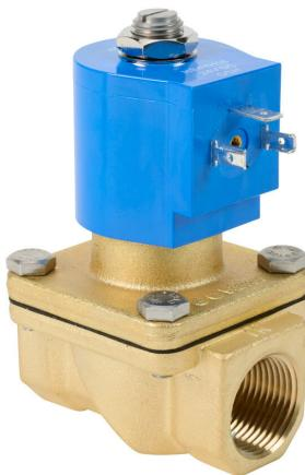
GC Valves solenoid valve, 2-port (2-way), 2-position, N.C., brass body, nitrile seal(s), 3/4in female NPT inlet(s), 3/4in female NPT outlet(s), Cv=6.7, 0 psi minimum operating pressure, 24 VDC operating voltage, 18mm DIN style wiring plug.
