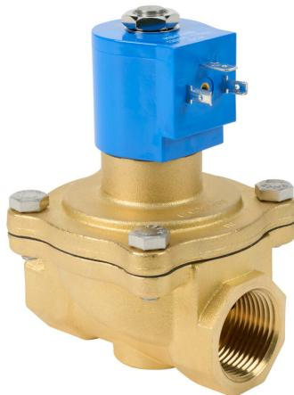
GC Valves solenoid valve, 2-port (2-way), 2-position, N.C., brass body, Viton seal(s), 1in female NPT inlet(s), 1in female NPT outlet(s), Cv=11, 0 psi minimum operating pressure, 120 VAC operating voltage, 18mm DIN style wiring plug.
