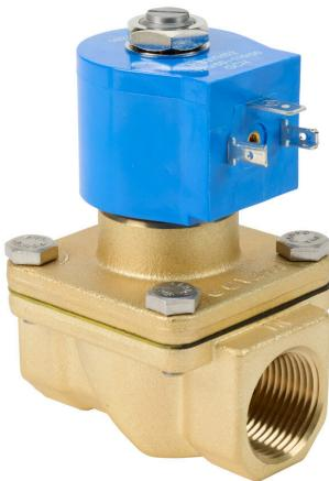
GC Valves solenoid valve, 2-port (2-way), 2-position, N.C., brass body, Viton seal(s), 3/4in female NPT inlet(s), 3/4in female NPT outlet(s), Cv=6.7, 0 psi minimum operating pressure, 120 VAC operating voltage, 18mm DIN style wiring plug.
