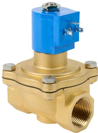
GC Valves solenoid valve, 2-port (2-way), 2-position, N.C., brass body, nitrile seal(s), 1in female NPT inlet(s), 1in female NPT outlet(s), Cv=11, 0 psi minimum operating pressure, 120 VAC operating voltage, 18mm DIN style wiring plug.
