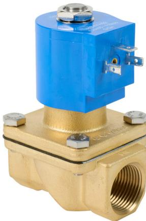
GC Valves solenoid valve, 2-port (2-way), 2-position, N.C., brass body, nitrile seal(s), 3/4in female NPT inlet(s), 3/4in female NPT outlet(s), Cv=6.7, 0 psi minimum operating pressure, 120 VAC operating voltage, 18mm DIN style wiring plug.
