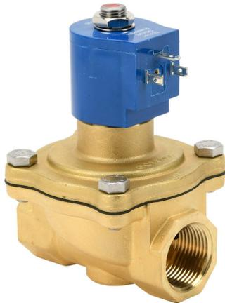
GC Valves solenoid valve, 2-port (2-way), 2-position, N.C., brass body, Viton seal(s), 1in female NPT inlet(s), 1in female NPT outlet(s), Cv=11, 0 psi minimum operating pressure, 24 VDC operating voltage, 18mm DIN style wiring plug.
