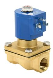
GC Valves solenoid valve, 2-port (2-way), 2-position, N.C., brass body, Viton seal(s), 1/2in female NPT inlet(s), 1/2in female NPT outlet(s), Cv=4.3, 0 psi minimum operating pressure, 24 VDC operating voltage, 18mm DIN style wiring plug.
