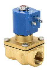
GC Valves solenoid valve, 2-port (2-way), 2-position, N.C., brass body, nitrile seal(s), 3/4in female NPT inlet(s), 3/4in female NPT outlet(s), Cv=6.7, 0 psi minimum operating pressure, 24 VDC operating voltage, 18mm DIN style wiring plug.
