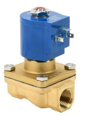
GC Valves solenoid valve, 2-port (2-way), 2-position, N.C., brass body, nitrile seal(s), 1/2in female NPT inlet(s), 1/2in female NPT outlet(s), Cv=4.3, 0 psi minimum operating pressure, 24 VDC operating voltage, 18mm DIN style wiring plug.
