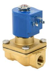
GC Valves solenoid valve, 2-port (2-way), 2-position, N.C., brass body, nitrile seal(s), 3/8in female NPT inlet(s), 3/8in female NPT outlet(s), Cv=4.3, 0 psi minimum operating pressure, 24 VDC operating voltage, 18mm DIN style wiring plug.
