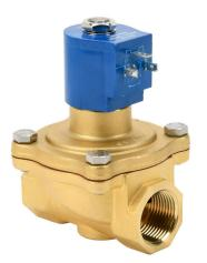
GC Valves solenoid valve, 2-port (2-way), 2-position, N.C., brass body, Viton seal(s), 1in female NPT inlet(s), 1in female NPT outlet(s), Cv=11, 0 psi minimum operating pressure, 120 VAC operating voltage, 18mm DIN style wiring plug.
