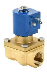
GC Valves solenoid valve, 2-port (2-way), 2-position, N.C., brass body, Viton seal(s), 3/4in female NPT inlet(s), 3/4in female NPT outlet(s), Cv=6.7, 0 psi minimum operating pressure, 120 VAC operating voltage, 18mm DIN style wiring plug.
