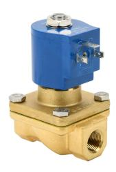
GC Valves solenoid valve, 2-port (2-way), 2-position, N.C., brass body, Viton seal(s), 3/8in female NPT inlet(s), 3/8in female NPT outlet(s), Cv=4.3, 0 psi minimum operating pressure, 120 VAC operating voltage, 18mm DIN style wiring plug.
