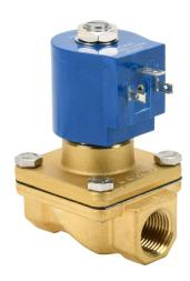
GC Valves solenoid valve, 2-port (2-way), 2-position, N.C., brass body, nitrile seal(s), 1/2in female NPT inlet(s), 1/2in female NPT outlet(s), Cv=4.3, 0 psi minimum operating pressure, 120 VAC operating voltage, 18mm DIN style wiring plug.
