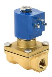
GC Valves solenoid valve, 2-port (2-way), 2-position, N.C., brass body, nitrile seal(s), 3/8in female NPT inlet(s), 3/8in female NPT outlet(s), Cv=4.3, 0 psi minimum operating pressure, 120 VAC operating voltage, 18mm DIN style wiring plug.
