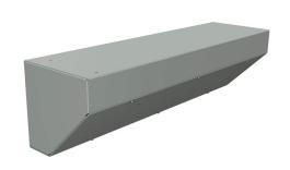
Wiegmann wiring trough, 10 x 10 x 36in (HxDxL), NEMA 1, corner mount, carbon steel, ANSI 61 gray, powder coat finish, screw cover.
