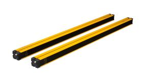
ReeR safety light curtain, sender/receiver pair, body protection, 24 VDC, 300mm resolution, 910mm protected height, 0-12m operating distance, safety category Type 4, IP65 IP67, (1) 5-pin and (1) 8-pin M12 quick-disconnect.
