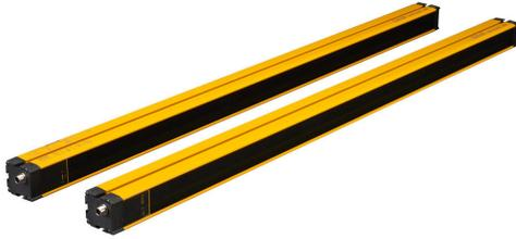
ReeR safety light curtain, sender/receiver pair, body protection, 24 VDC, 300mm resolution, 910mm protected height, 0-12m operating distance, safety category Type 4, IP65 IP67, (1) 5-pin and (1) 8-pin M12 quick-disconnect.
