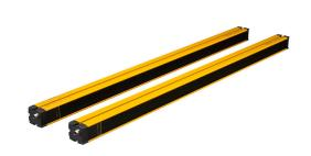
ReeR safety light curtain, sender/receiver pair, body protection, 24 VDC, 300mm resolution, 910mm protected height, 0-12m operating distance, safety category Type 4, IP65 IP67, (1) 5-pin and (1) 8-pin M12 quick-disconnect.
