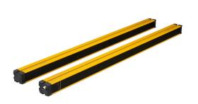
ReeR safety light curtain, active/passive pair, body protection, 24 VDC, 300mm resolution, 910mm protected height, 0-8m operating distance, safety category Type 4, IP65 IP67, (1) 8-pin M12 quick-disconnect.
