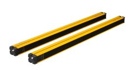
ReeR safety light curtain, sender/receiver pair, body protection, 24 VDC, 400mm resolution, 810mm protected height, 0-12m operating distance, safety category Type 4, IP65 IP67, (1) 5-pin and (1) 8-pin M12 quick-disconnect.
