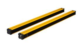
ReeR safety light curtain, active/passive pair, body protection, 24 VDC, 400mm resolution, 810mm protected height, 0-8m operating distance, safety category Type 4, IP65 IP67, (1) 8-pin M12 quick-disconnect.
