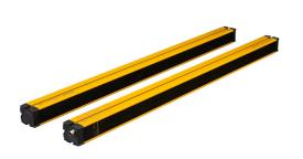
ReeR safety light curtain, active/passive pair, body protection, 24 VDC, 400mm resolution, 810mm protected height, 0-8m operating distance, safety category Type 4, IP65 IP67, (1) 8-pin M12 quick-disconnect.
