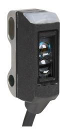
ProSense photoelectric sensor, rectangular, diffuse, visible red, 180mm sensing distance, light-on, PNP, 1000 Hz switching frequency, ABS plastic housing, 4-pin M8 quick-disconnect.
