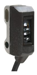
ProSense photoelectric sensor, rectangular, diffuse, visible red, 180mm sensing distance, light-on, PNP, 1000 Hz switching frequency, ABS plastic housing, pigtail.
