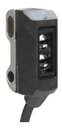
ProSense photoelectric sensor, rectangular, diffuse with background suppression, 1-80mm sensing distance, light-on, PNP, 1000 Hz switching frequency, 11.8in/300mm cable length, 4-pin M8 quick-disconnect.
