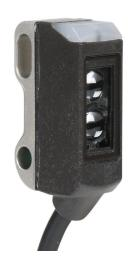
ProSense photoelectric sensor, rectangular, diffuse with background suppression, 1-80mm sensing distance, light-on, PNP, 1000 Hz switching frequency, 6.5ft/2m cable length, pigtail.
