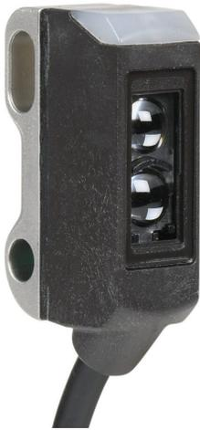
ProSense photoelectric sensor, rectangular, diffuse with background suppression, 1-50mm sensing distance, light-on, PNP, 1000 Hz switching frequency, 11.8in/300mm cable length, 4-pin M8 quick-disconnect.
