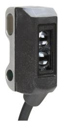
ProSense photoelectric sensor, rectangular, diffuse with background suppression, 1-50mm sensing distance, light-on, PNP, 1000 Hz switching frequency, 11.8in/300mm cable length, 4-pin M8 quick-disconnect.
