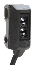
ProSense photoelectric sensor, rectangular, diffuse with background suppression, 1-50mm sensing distance, light-on, PNP, 1000 Hz switching frequency, 6.5ft/2m cable length, pigtail.
