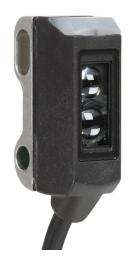
ProSense photoelectric sensor, rectangular, diffuse with background suppression, 3-15mm sensing distance, light-on, PNP, 1000 Hz switching frequency, 11.8in/300mm cable length, 4-pin M8 quick-disconnect.
