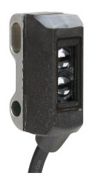
ProSense photoelectric sensor, rectangular, diffuse with background suppression, 1-80mm sensing distance, light-on, NPN, 1000 Hz switching frequency, 11.8in/300mm cable length, 4-pin M8 quick-disconnect.
