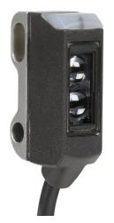
ProSense photoelectric sensor, rectangular, diffuse with background suppression, 3-15mm sensing distance, light-on, NPN, 1000 Hz switching frequency, 11.8in/300mm cable length, 4-pin M8 quick-disconnect.
