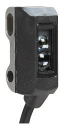
ProSense photoelectric sensor, rectangular, ABS plastic housing, through-beam receiver, 3m sensing distance, 10-30 VDC operating voltage, dark-on, PNP, 3-wire, 4-pin M8 quick-disconnect.
