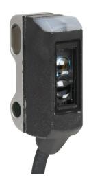
ProSense photoelectric sensor, rectangular, ABS plastic housing, through-beam receiver, visible red light emission, 3m sensing distance, 10-30 VDC operating voltage, dark-on, PNP, 3-wire, pigtail.
