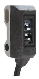
ProSense photoelectric sensor, rectangular, ABS plastic housing, through-beam receiver, 3m sensing distance, 10-30 VDC operating voltage, dark-on, NPN, 3-wire, 4-pin M8 quick-disconnect.
