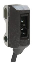
ProSense photoelectric sensor, rectangular, polarized retroreflective, visible red light emission, 0.02-1.8m sensing distance, dark-on, PNP, 3-wire, pigtail.
