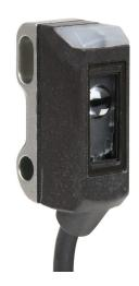
ProSense photoelectric sensor, rectangular, ABS plastic housing, through-beam emitter, visible red light emission, 3m sensing distance, 10-30 VDC operating voltage, 2-wire, pigtail.
