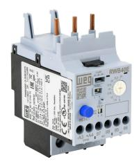
WEG Electric RWB40E series electronic overload relay, 5–25.0A adjustable, solid state, remote/local reset, direct mount power connection(s). For use with CWB9 to CWB38 and CWBN00 to CWBN1series contactors.
