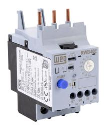
WEG Electric RWB40E series electronic overload relay, 1.6-8.0A adjustable, solid state, direct mount power connection(s). For use with CWB9 to CWB38 series contactors.
