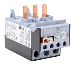
WEG Electric RW67-5D series thermal overload relay, 57.0-70.0A adjustable, bi-metallic, direct mount power connection(s). For use with CWB40 to CWB80 series contactors.
