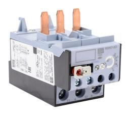
WEG Electric RW67-5D series thermal overload relay, 50.0-63.0A adjustable, bi-metallic, direct mount power connection(s). For use with CWB40 to CWB80 series contactors.
