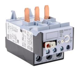
WEG Electric RW67-5D series thermal overload relay, 40.0-57.0A adjustable, bi-metallic, direct mount power connection(s). For use with CWB40 to CWB80 series contactors.
