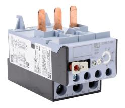
WEG Electric RW67-5D series thermal overload relay, 32.0-50.0A adjustable, bi-metallic, direct mount power connection(s). For use with CWB40 to CWB80 series contactors.
