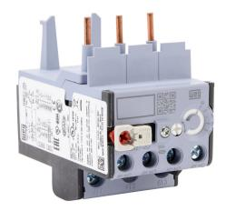
WEG Electric RW27-2D series thermal overload relay, 32.0-40.0A adjustable, bi-metallic, direct mount power connection(s). For use with CWB9 to CWB38 series contactors.
