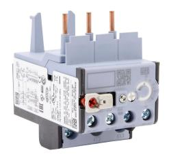
WEG Electric RW27-2D series thermal overload relay, 22.0-32.0A adjustable, bi-metallic, direct mount power connection(s). For use with CWB9 to CWB38 series contactors.
