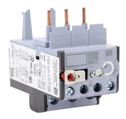
WEG Electric RW27-2D series thermal overload relay, 7.0-10.0A Adjustable, bi-metallic, direct mount power connection(s). For use with CWB9 to CWB38 series contactors.
