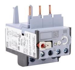
WEG Electric RW27-2D series thermal overload relay, 5.6-8.0A Adjustable, bi-metallic, direct mount power connection(s). For use with CWB9 to CWB38 series contactors.
