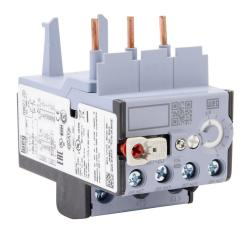
WEG Electric RW27-2D series thermal overload relay, 2.8-4.0A Adjustable, bi-metallic, direct mount power connection(s). For use with CWB9 to CWB38 series contactors.
