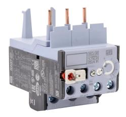
WEG Electric RW27-2D series thermal overload relay, 8.0-12.5A Adjustable, bi-metallic, direct mount power connection(s). For use with CWB9 to CWB38 series contactors.
