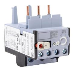
WEG Electric RW27-2D series thermal overload relay, 1.8-2.8A adjustable, bi-metallic, direct mount power connection(s). For use with CWB9 to CWB38 series contactors.
